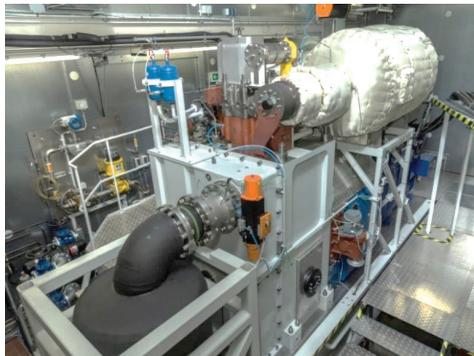
*Figure 6: View on SCE 34 DF Engine in Test Bed*
