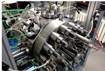
*Figure 3: Section of the CAD Model of the High Pressure – High Temperature Chamber (left) and Photograph of the Chamber and Measurement System (right)*
