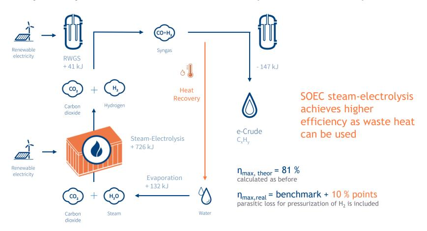
All values refer to energy conversion necessary for the production of 1 kmol of -CxHy- hydrocarbons RWGS: Reverse-Water-Gas-Shift-Reaction
