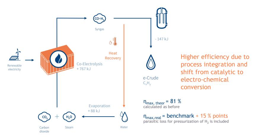
All values refer to energy conversion necessary for the production of 1 kmol of -CxHy- hydrocarbons RWGS: Reverse-Water-Gas-Shift-Reaction
