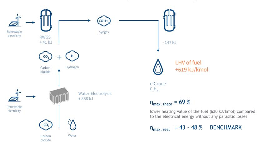
All values refer to energy conversion necessary for the production of 1 kmol of -CxHy- hydrocarbons
